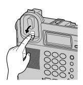
**2** Press the tabs in the direction of the arrows (1), then remove the wall mounting adaptor (2).
